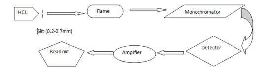
\3. In the schematic diagram of AAS where is the slit being placed?
